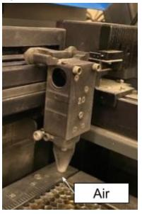
If you do not feel a steady stream of air out the hole in the bottom of the cutting head, **do not continue with cutting** and contact us immediately.
